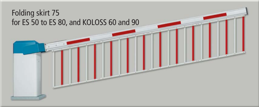
Folding skirt 75, flat-rolled aluminium, 15x3mm, white or red/white, 750mm high, weight: 1.5kg/m
